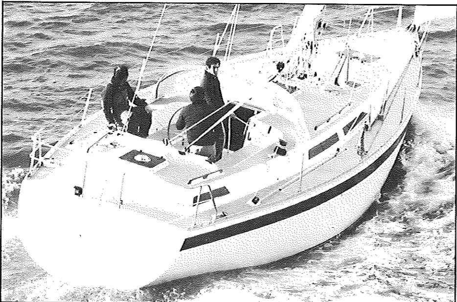
Deck has a clean profile for a centre cockpit yacht. Good non-slip and clean side decks allow easy movement. Starboard genoa sheet cleat needs re-positioning to prevent the sheet from fouling itself
