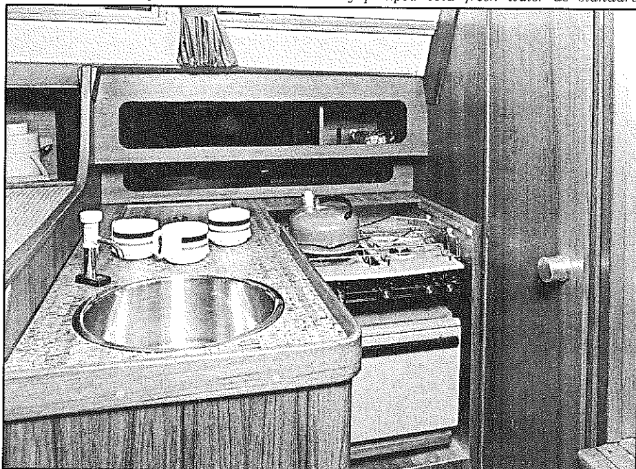
The galley is compact, but easy to work and there is plenty of stowage for consumables. The circular sink is deep and served with manually pumped cold fresh water as standard
