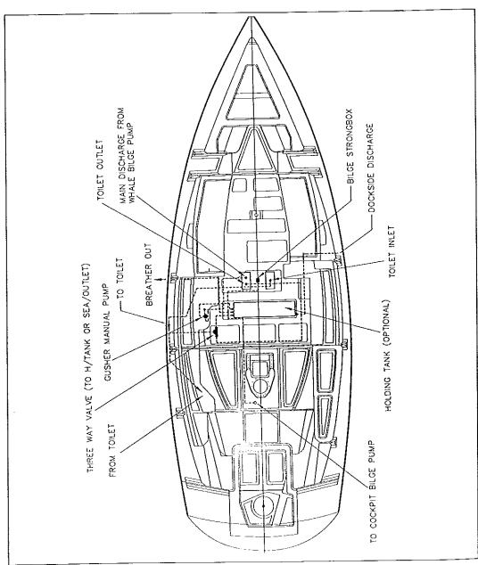
The hull of the Moody 36 contains a single bilge compartment, serviced by a hand-operated bilge pump located in the portside of the cockpit (an electric bilge pump is provided as an optional extra).
