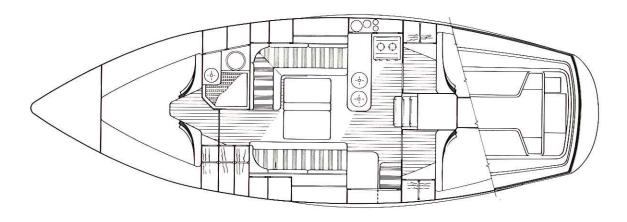
**General:** Hull and superstructure in GRP to Lloyds specification. 8 berth 4 cabins, aft cockpit, sloop rig, diesel inboard engine, separate toilet compartment with shower.
